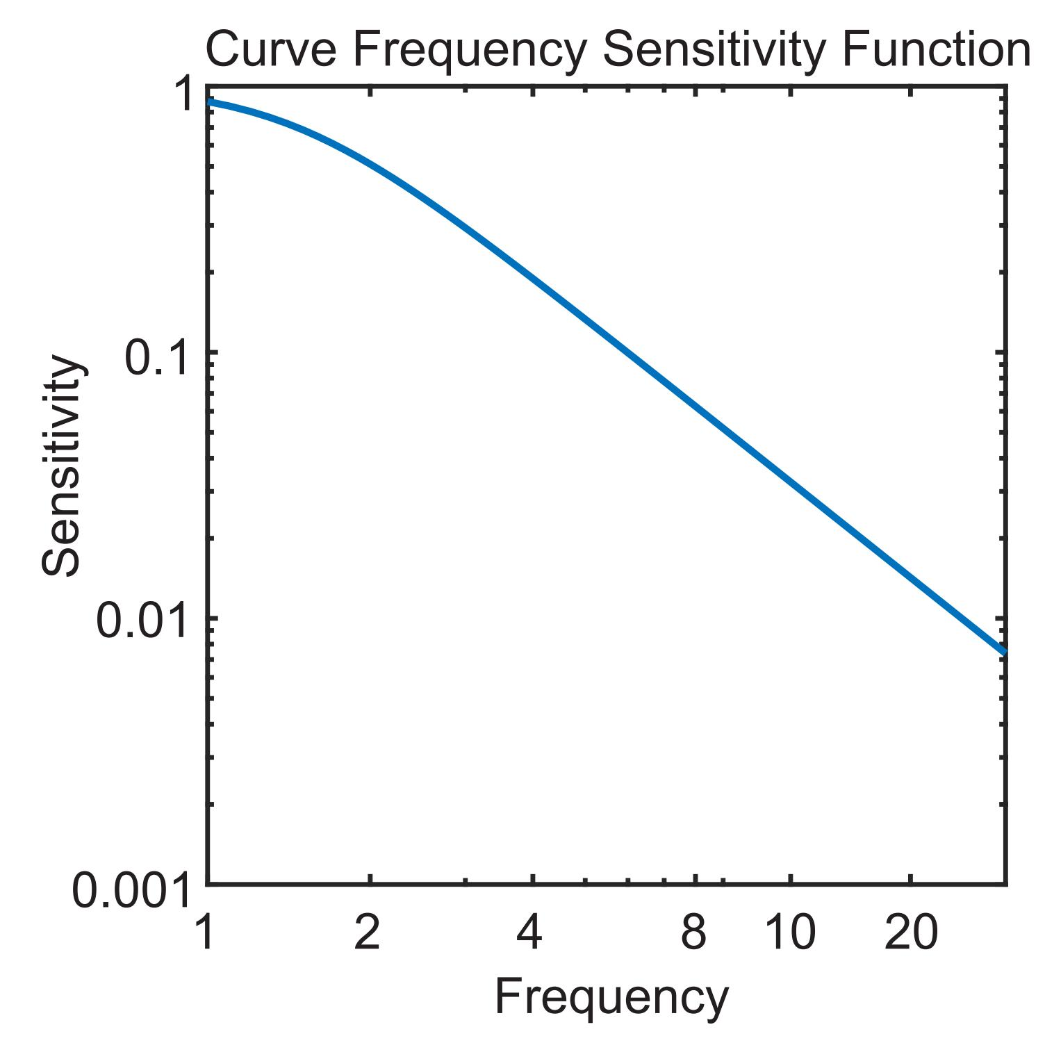
The model assumes a Curve Frequency Sensitivity Function (CSFF), which is characterized by a flat followed by declining response (sensitivity) to curvature as a function of modulation frequency. The decline in response to curvature at high modulation frequencies embodies the idea of a perceptual limitation for high curve frequencies.
